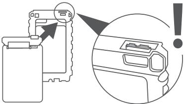
**EN** Wrap the inner rubber shock absorber around the SSD/HDD and SATA adapter assembly. Make sure the One Touch Auto-backup button and the USB connector on the SATA adapter are exposed and unobstructed.
